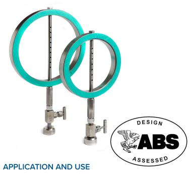
When using the DREW Bunker Sampler, sampling is carried out by continuous drip during the entire bunkering period. A valve on the sampler is used to adjust the drip rate into either the 5 L or 10 L Cubitainer receptacle connected to the sampler. A new Cubitainer should be used for each bunkering and each different grade of fuel.
